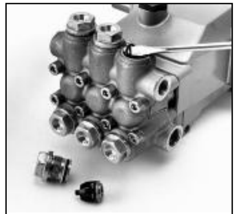
All Models Removal of Valve Seat O-Ring
